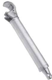
CLP-528L weight = 0,980 kg Quick release claw (51 mm) Max. allowable load 30 kg with expendable CCS6 Working length 320-345 mm
