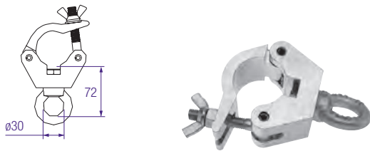
CLP-537 weight = 0,830 kg Clamp (48-51 mm) With eye-nut M12 SVWL 340 kg
