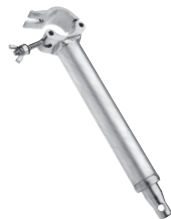
CLP-529L weight = 1,210 kg Clamp (48-51 mm) Max. allowable load 35 kg with expendable CCS6 Working length 320-345 mm
