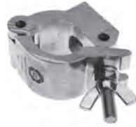
CLP-587 weight = 0,570 kg Side entry clamp (48-51 mm) SVWL 750 kg
