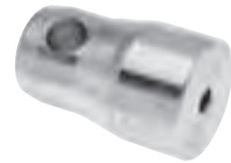
CCS4-402 weight = 0,050 kg Offset half conical coupler | Offset 15 mm, thread M6
